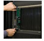
The Network I/O enclosure provides X.25 and X.29 communication
