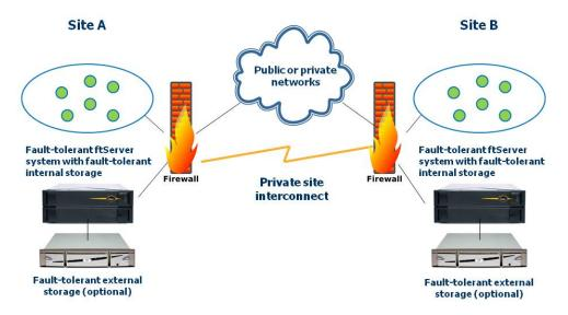
Figure 2: ACI active/active dual-site implementation using Stratus fault tolerance
